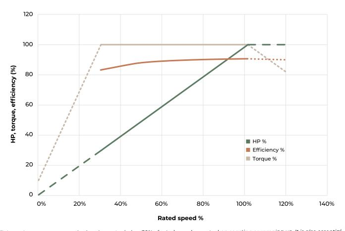
Infinitum does not recommend using the motor below 30% of rated speed except when coasting or ramping up. It is also essential to restrict power and FLA within the nameplate rating when operating the motor above 100% of its rated speed. If requiring rated speeds outside of the operating range, please contact the factory and our Application Engineers will provide a customized solution.
