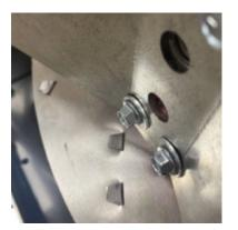
There are no adjustment slots on bent metal cube assemblies.
