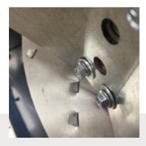
There are no adjustment slots on bent metal cube assemblies.
