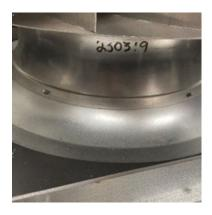
Each bent metal supporting piece has four holes that align with the Aircore EC motor mounting points.
